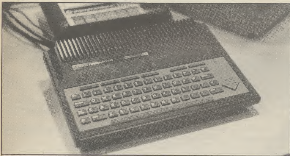
This is a little beastie you definitely won't see in any British shops. Called the Commodore 116, it's really a Commodore 16 with a small Plus/4-style case and 'chiclet' keys rather like the old Spectrum. Apparently the machine was to be marketed only in Germany where it hasn't gone down very well. Yet another black mark for Commodore's marketing strategy.
